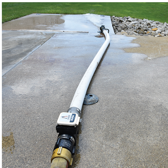
AkroFlow Portable Flow Meter connected to fire hose
