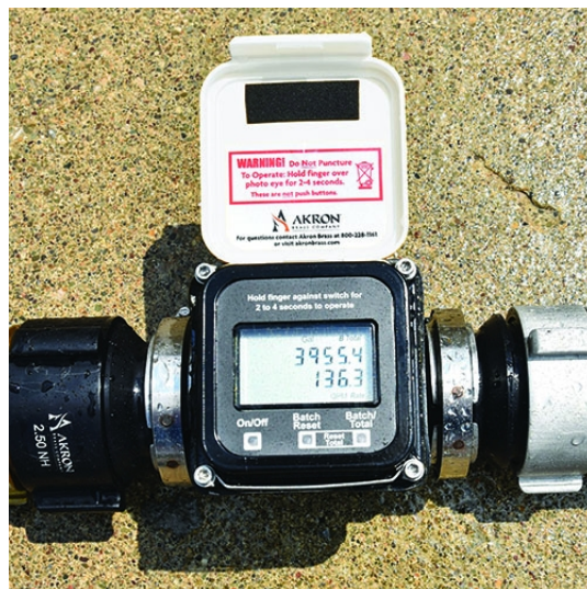
Display on AkroFlow Portable Flow Meter
