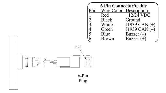
Figure 3. Wiring
