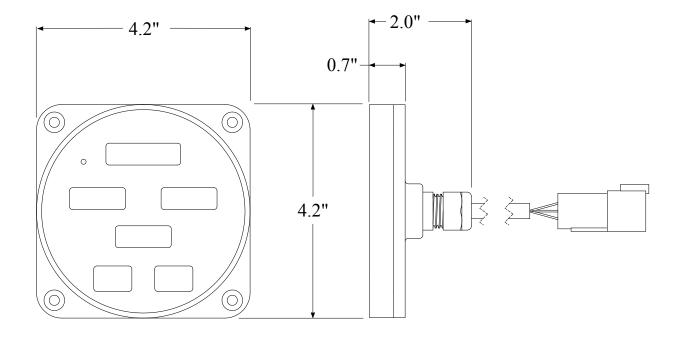
Figure 2. Display Module Mounting Dimensions
