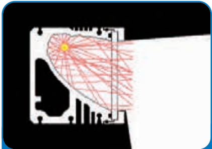
A cross section of the FOCUS lamphead showing its unique reflector surfaces that redirect light waves for even, bright scene lighting where it's most needed.
